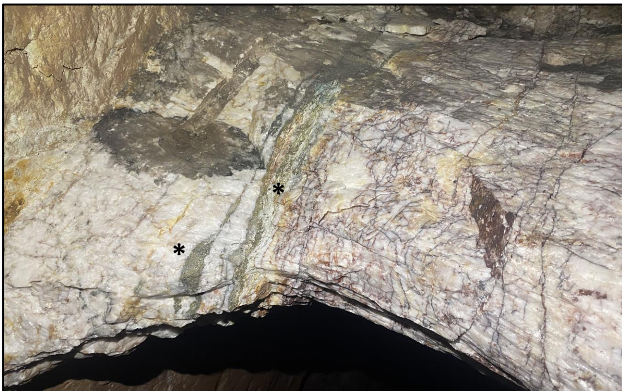
Figure 4: MVZ quartz vein underground, showing lenses and ribbons of vein-parallel sulphidic material (*)
