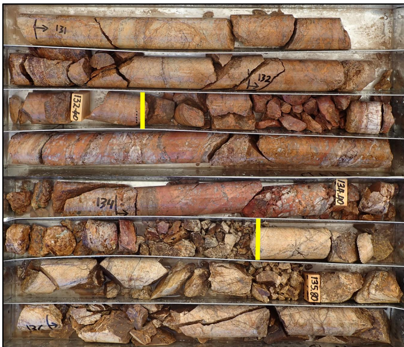
Figure 5: Uncut drill core from hole AMD-108, 130.97m to 136.61m depth, showing the Fin Vein mineralised zone between 132.50m and 135.00m
